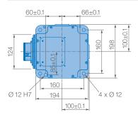
Mounting options: Floor, ceiling, wall, tilt\* Protection class: IP67
