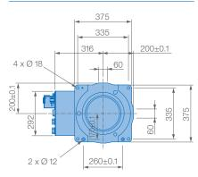
Mounting options: Floor, ceiling, wall Protection class: IP54/67
